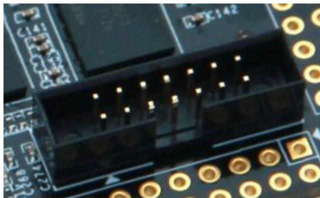
Figure 4-4: The JTAG on the FPGA Core Board
