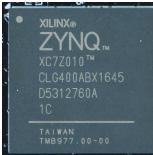
Figure 4-2: The XC7Z010 chip on the Core Board AC7010
