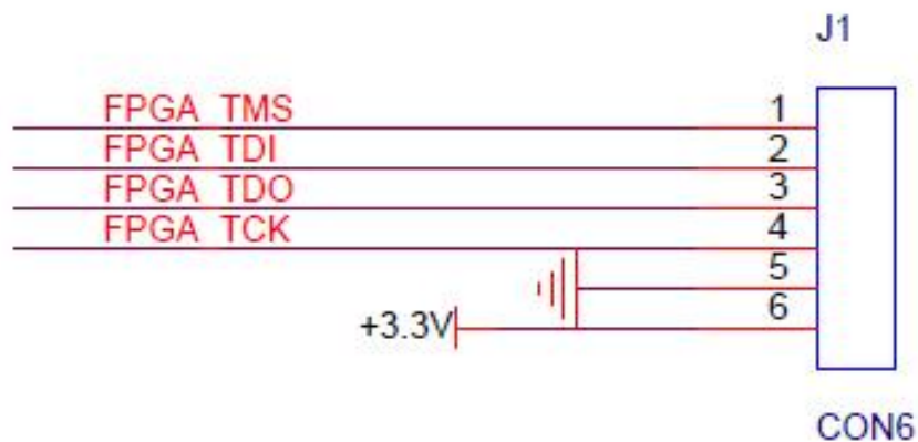
Figure 8-1: JTAG Interface Schematic
