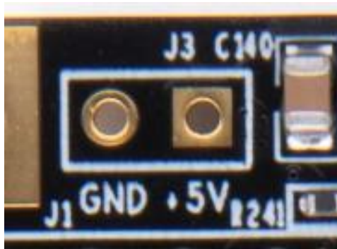
Figure 9-1: Power Interface on the Core Board
