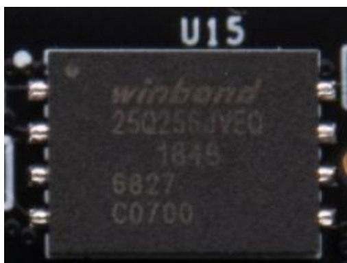
Figure 1-4-2: QSPI Flash on the core board
