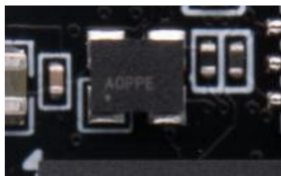
Figure 1-5-2: 33.333333Mhz active crystal on the core board
