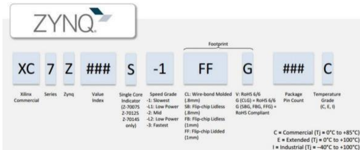
Figure 1-2-2: The Specific Chip Model Definition of ZYNQ7000 Series
