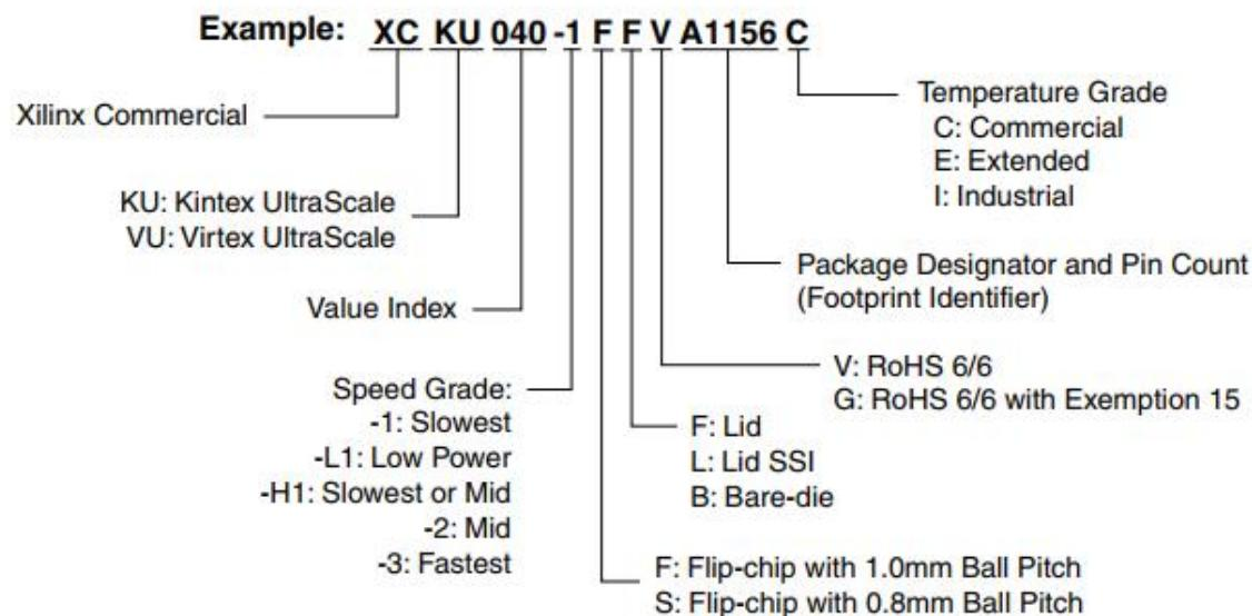
Figure 1-2-1 Definition of Xilinx's KINTEX UltraSacale series
