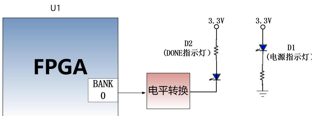
Table1-6-1 LED lights on core board Schematic
