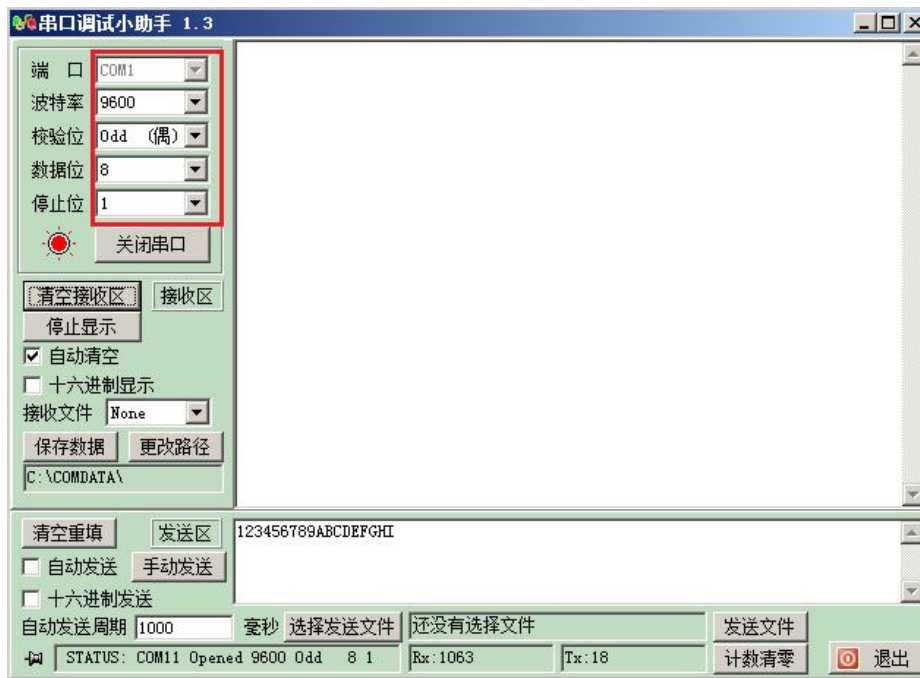
Figure 3-3: The Specific Configuration of Serial Debugging Assistant
