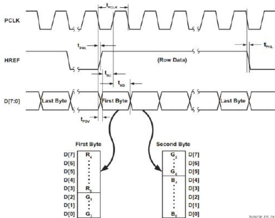
Figure 3-3: RGB 585 Output Timing Diagram
