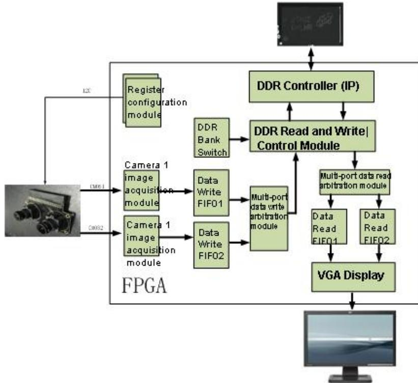
Figure 4-1: The logic block diagram of the FPGA program
