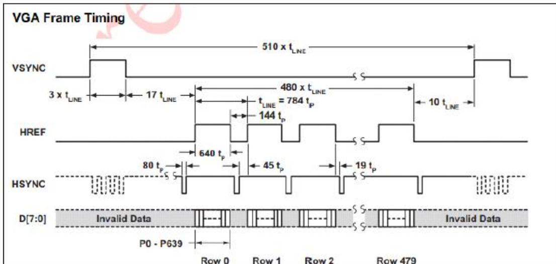
Figure 2-2: VGA Frame Timing
