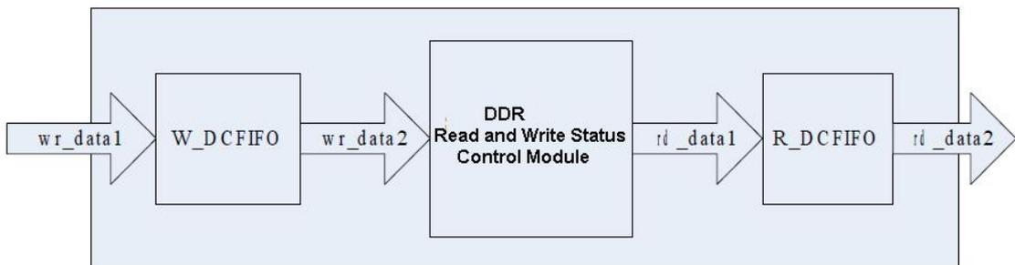
Figure 3-4: FIFO Control Program Module
