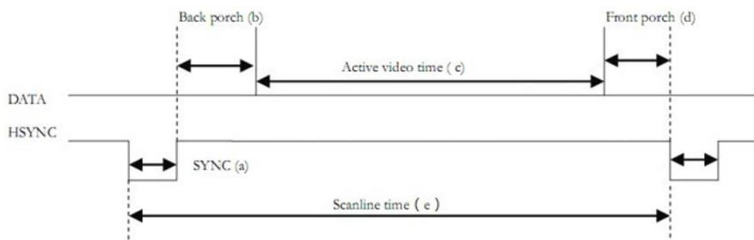
Figure 3-8: VGA Time Timing
