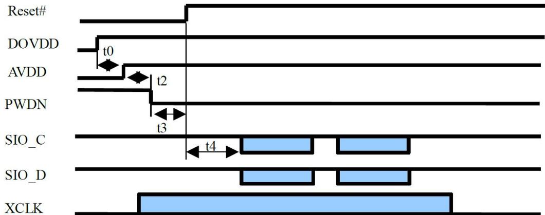
$t_0$ :  $\geq 0$ ms. Delay from DOVDD stable to AVDD stable
