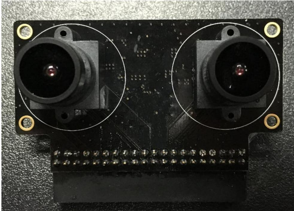
Figure 2-1: 40-pin Female header of Camera Module
