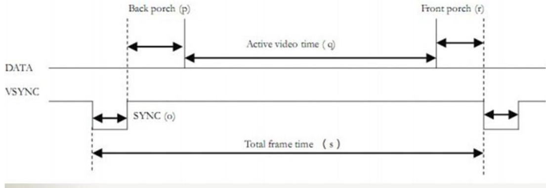
Figure 3-9: VGA Filed Timing
