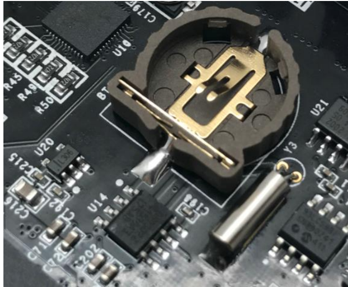
Figure 7-8: Real time clock DS1302 on the FPGA Board
