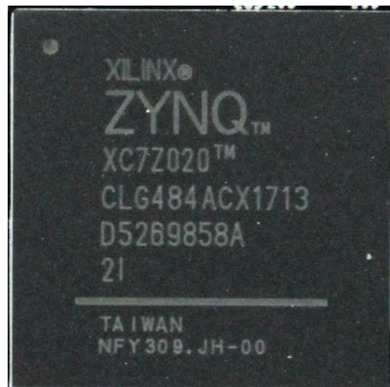
Figure 2-2: The Specific Chip Model Definition of ZYNQ7000 Series
