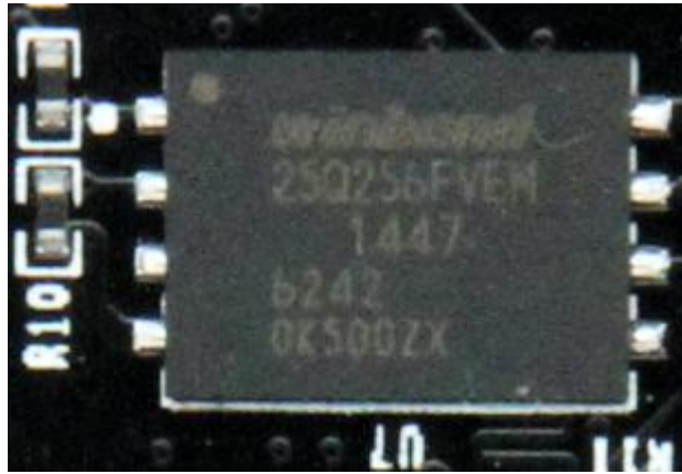
Figure 4-2: QSPI Flash on the Core Board
