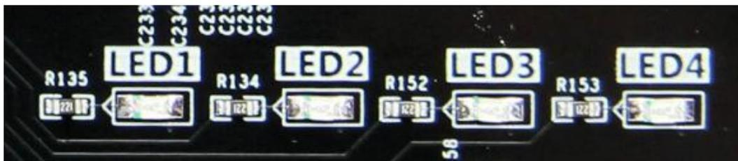
Figure 3-13-2: The User LEDs on the Carrier board
