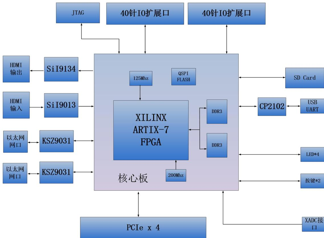
Figure 1-1-1: The Schematic Diagram of the AX7103
