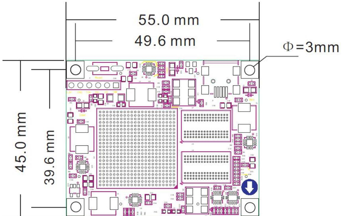
Figure 2-12-1: AC7100B FPGA Core board (Top view)
