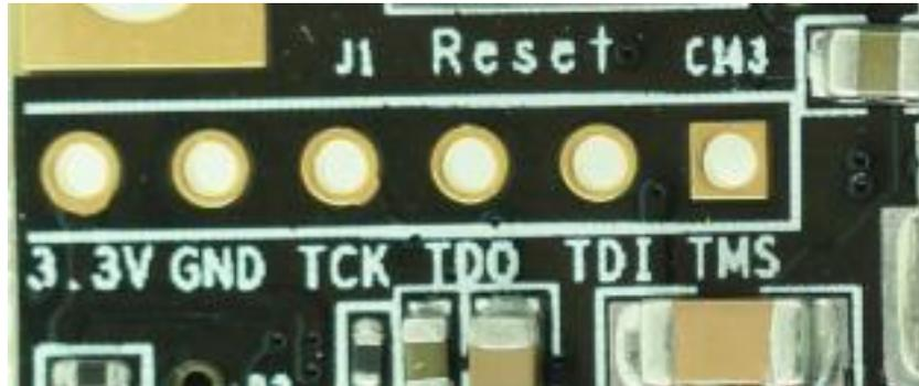
Figure 2-8-2: JTAG Interface on Core Board
