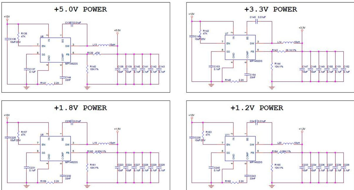
Figure 3-14-2: Power supply Schematic on the Carrier board
