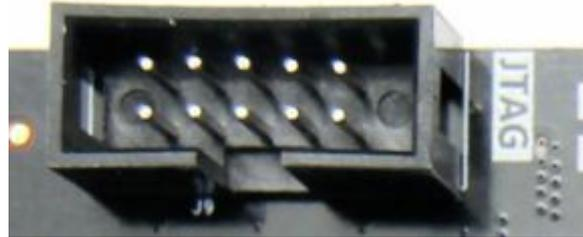
Figure 3-10-2: JTAG Interface on the carrier board
