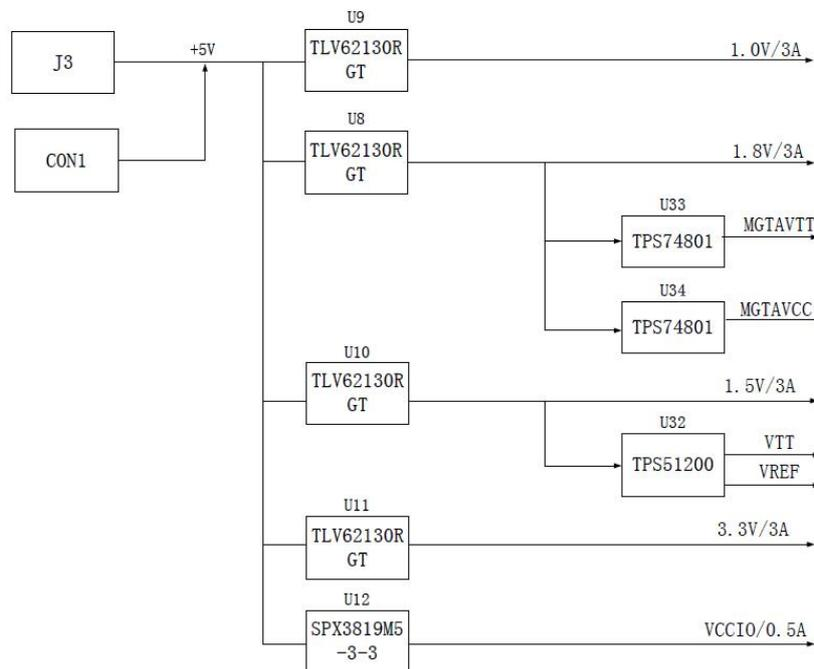
Figure 2-11-1: Power Supply on core board schematic
