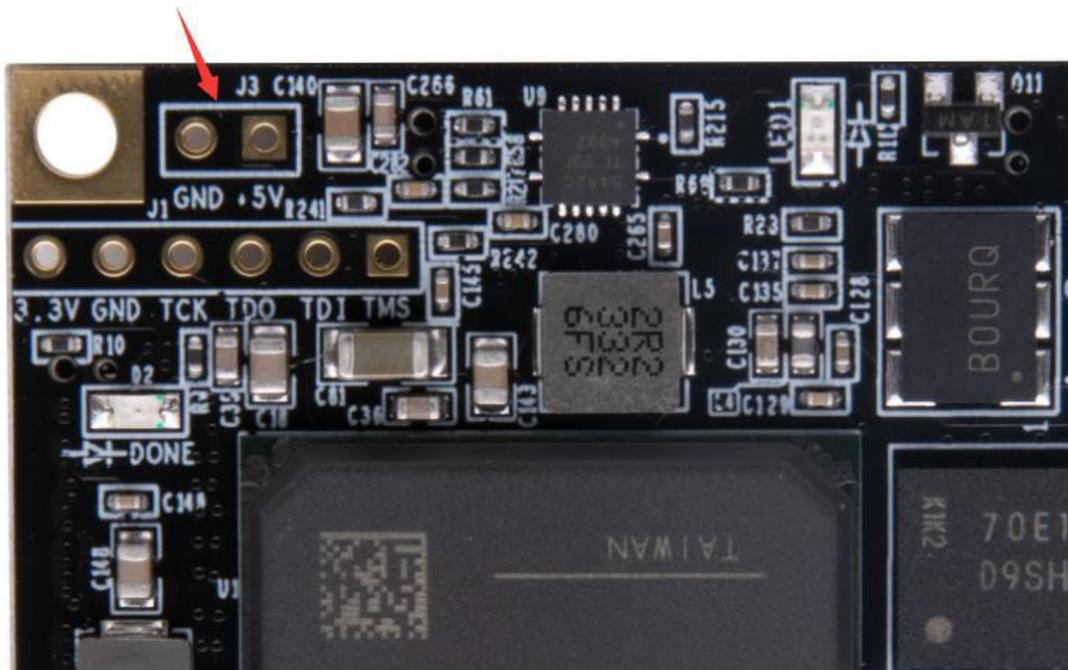
Figure 2-9-2: J3 interface on the Core Board
