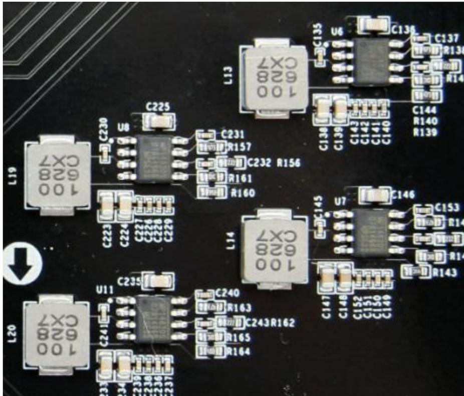
Figure 3-14-3: Power Supply Circuit on the Carrier board
