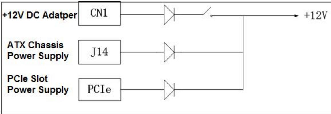
Figure 3-14-1: Power supply method for AX7103 FPGA Board
