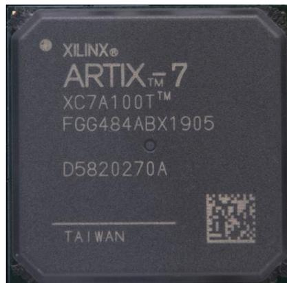
Figure 2-2-2: FPGA chip on board
