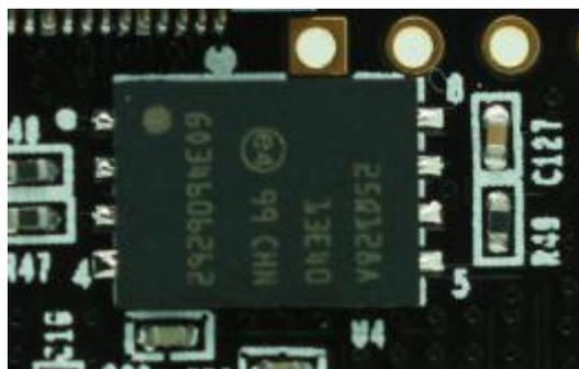
Figure 2-5-2: QSPI on the Core Board
