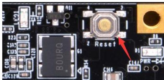
Figure 2-7-2: Reset key on the Core Board
