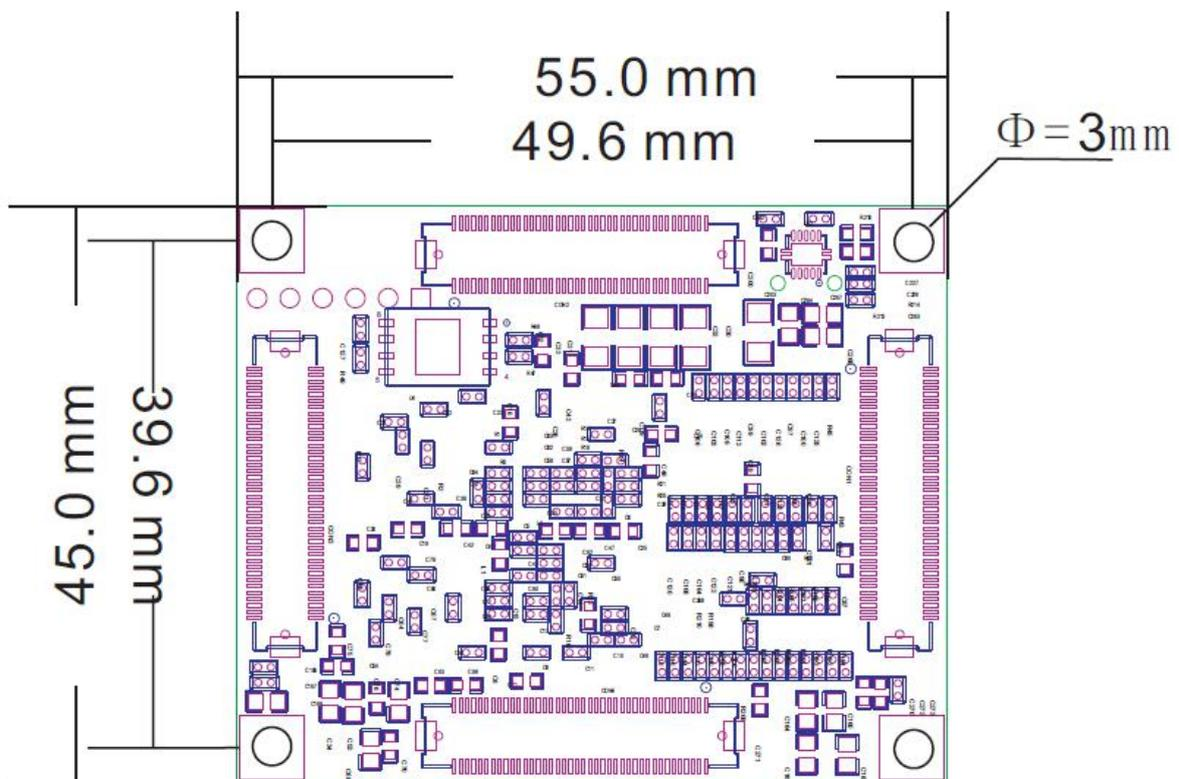
Figure 2-12-2: AC7100B FPGA Core board (Bottom view)
