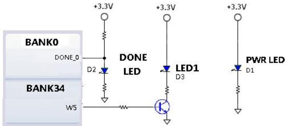
Figure 2-6-1: LED lights on core board Schematic
