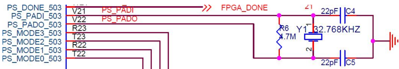
Figure 2-6-2: Passive Crystal Oscillator for RTC
