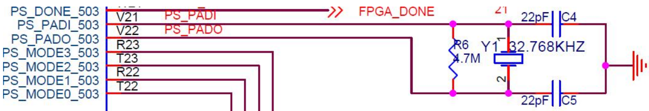
Figure 2-6-2: Passive Crystal Oscillator for RTC
