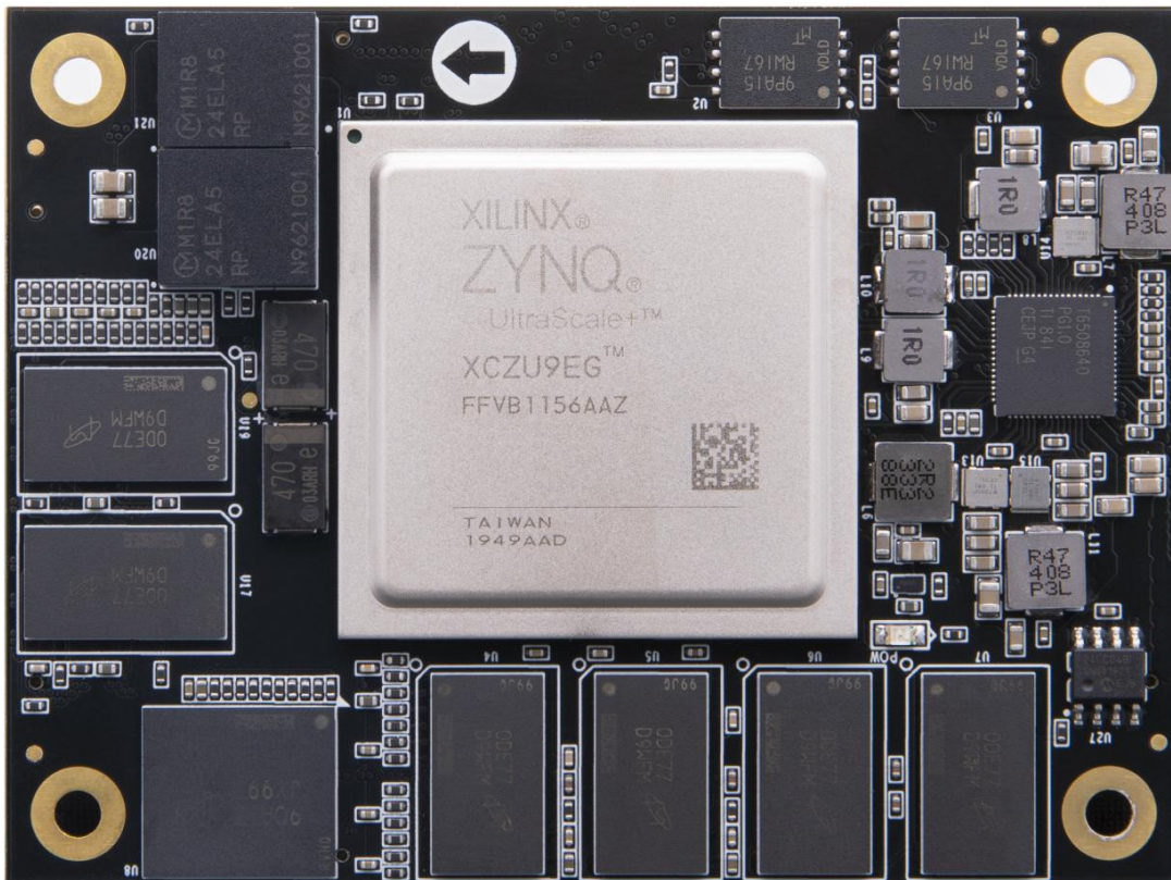
Figure 2-1-1: ACU9EG Core Board (Front View)
